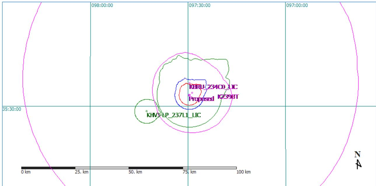
The green contours represent co-channel interfering (40 dBu) to co-channel protected (60 dBu) contours. Blue contours represent first-adjacent channel interfering (54 dBu) to first-adjacent protected (60 dBu) contours. Magenta contours represent second and third-adjacent channel interfering (100 dBu) to second and third-adjacent protected (60 dBu) contours. Red contours represent co-channel protected (60 dBu) to co-channel interfering (40 dBu) contours.
