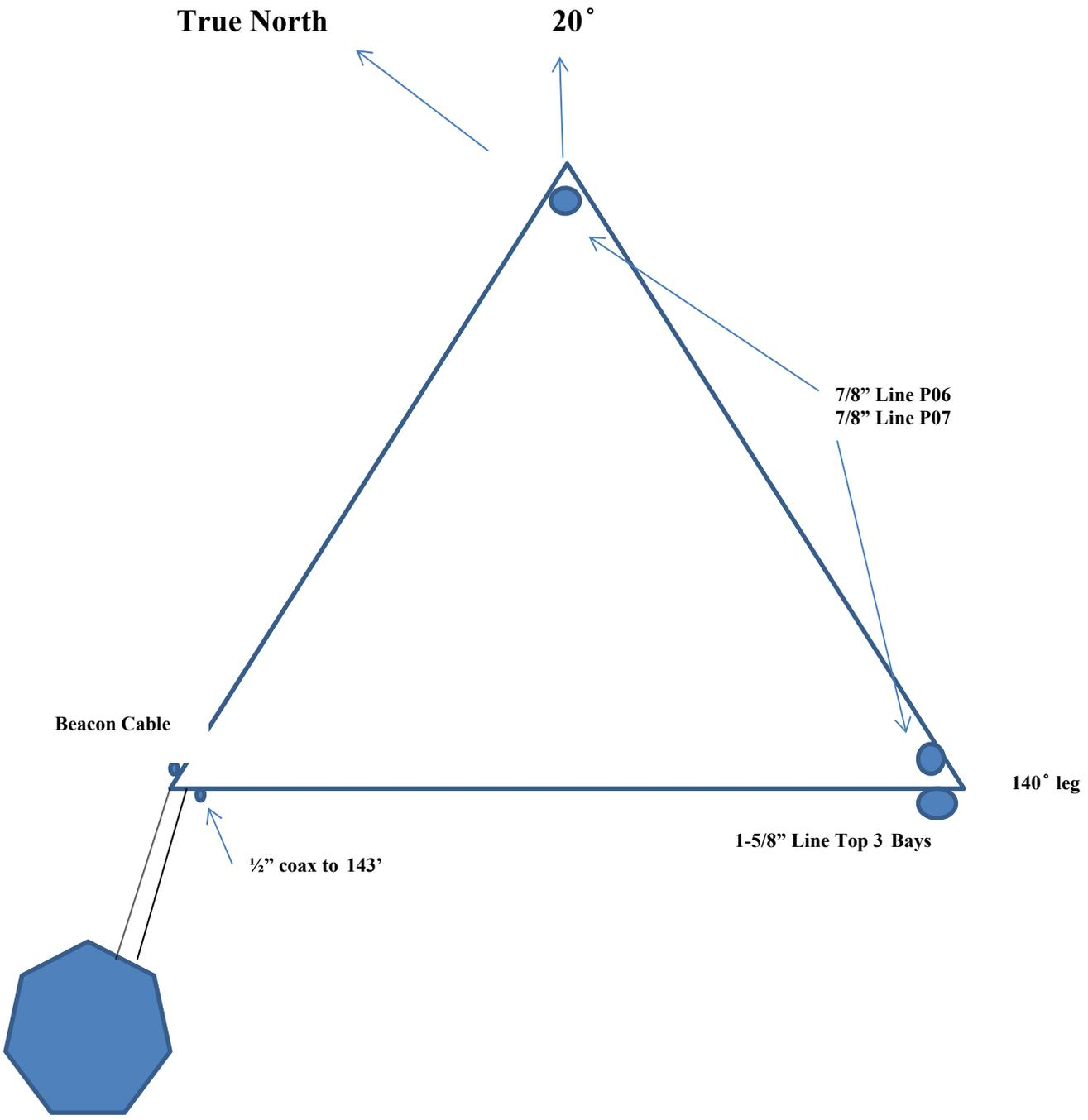
**Sketch showing where 7/8" line was installed for tests**
