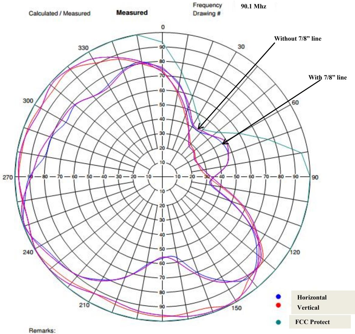
**Horizontal and vertical polarizations with and without additional 7/8" line.
