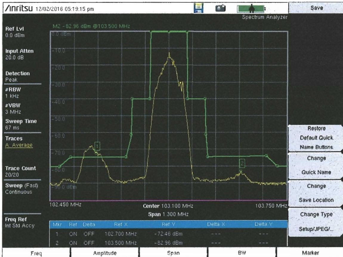
Note: The signals at 102.7 MHz and 103.5 MHz are from other nearby stations and NOT a product of the stations being measured
