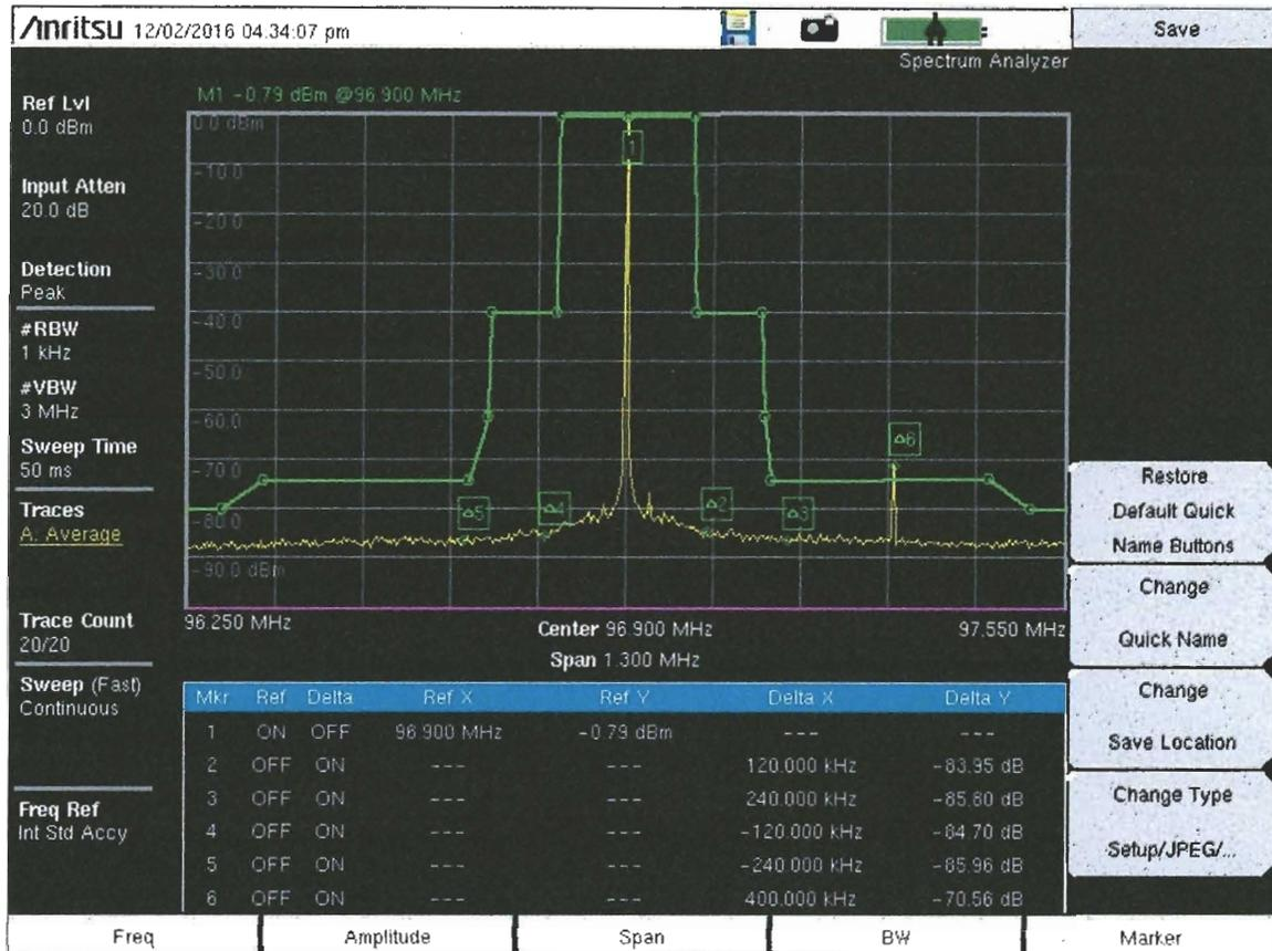
Note: The signal at + 400 KHz is from another signal at this site and NOT a product of the stations being measured
