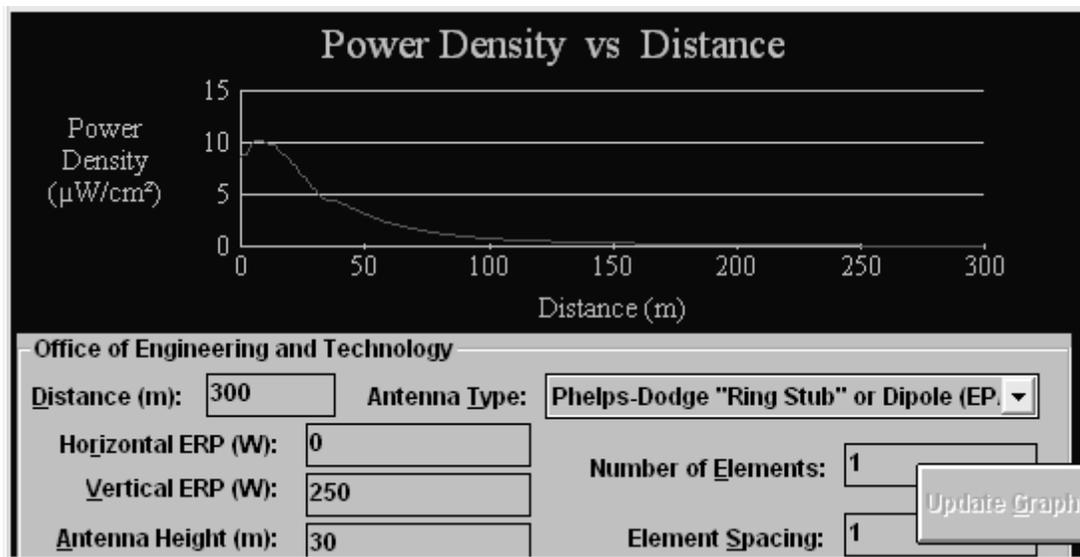
The Max Power Density was found to be 10.1517392084136  $\mu\text{W}/\text{cm}^2$  at 6 meters.
