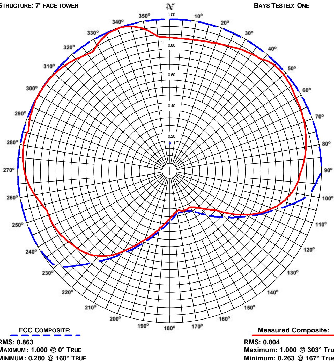
COMMENTS: COMPOSITE PATTERN: THIS PATTERN SHOWS THE MAXIMUM OF EITHER THE H OR V AZIMUTH VALUES. THIS PATTERN IS GREATER THAT 85% OF THE FCC FILED COMPOSITE PATTERN BPH-200251018AAX
