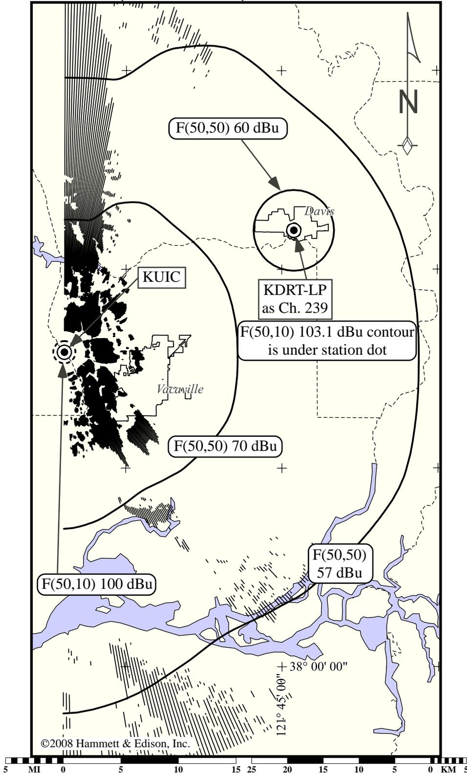
Lambert conformal conic map projection. Shadowing based upon 3-second USGS digitized terrain data and 4/3 earth radius, 9.1 m AGL RX height. Map data taken from Sectional Aeronautical Charts, published by the National Ocean Survey. Geographic coordinate marks shown at 15-minute increments. City limits shown taken from U.S. Census Bureau TIGER/Line 2000 data.
