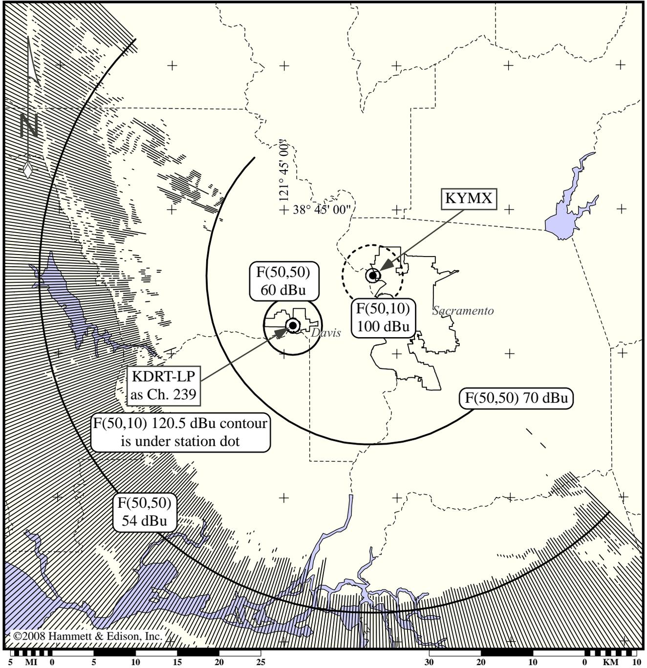
Lambert conformal conic map projection. Shadowing based upon 3-second USGS digitized terrain data and 4/3 earth radius, 9.1 m AGL RX height. Map data taken from Sectional Aeronautical Charts, published by the National Ocean Survey. Geographic coordinate marks shown at 15-minute increments. City limits shown taken from U.S. Census Bureau TIGER/Line 2000 data.
