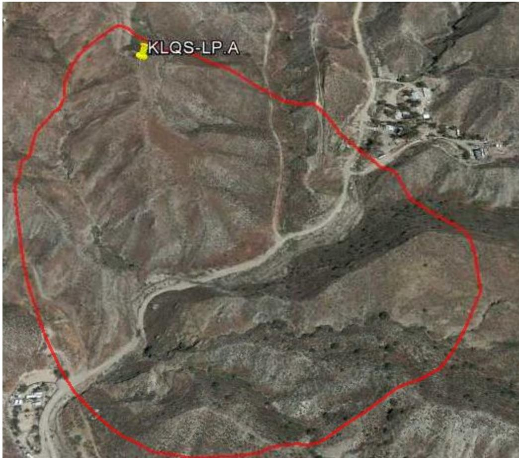
The red line delineates the interference area. This contour was generated via V-Soft FM Commander software and outputted to a Google Earth kml file. No population exists within the interference.
