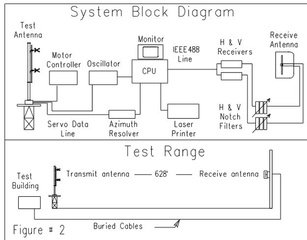
of radiation of the test approximately 30 feet above ground. The turntable is equipped with a motor drive and a US Digital angle position indicator. The resolution of this angle position indicator is one-hundredth of a degree.
