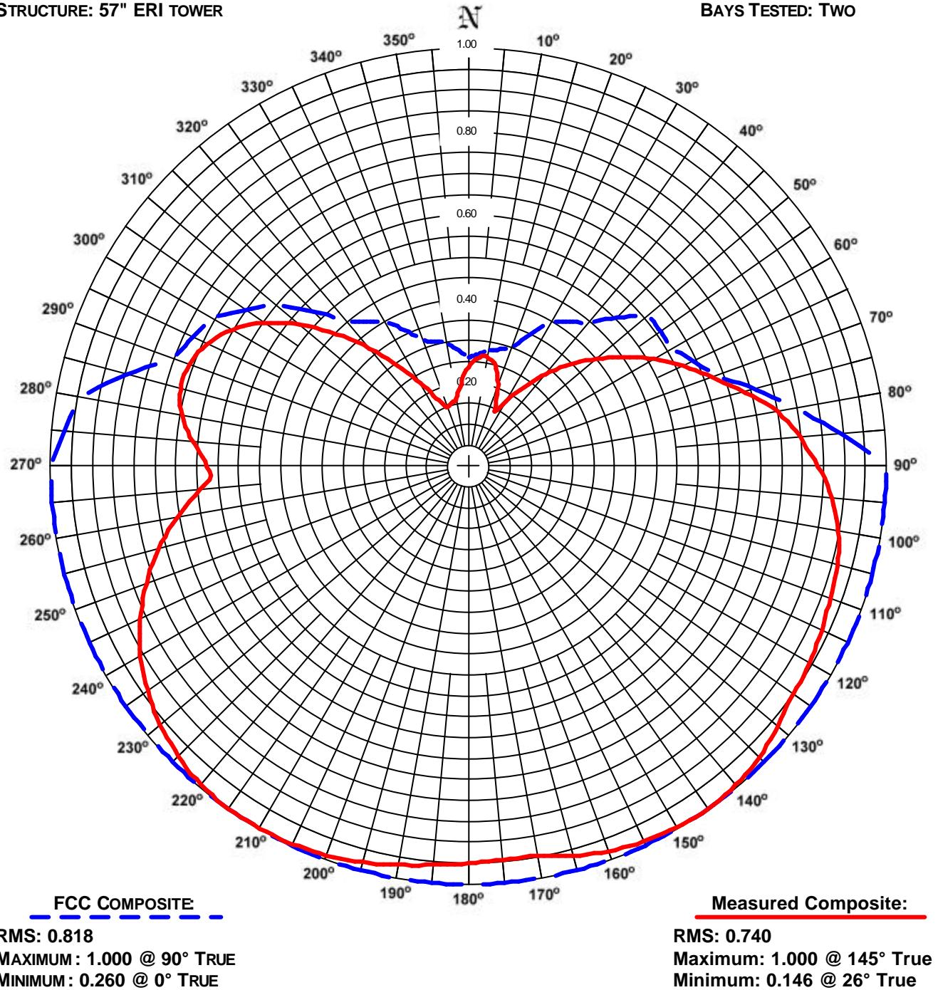
COMMENTS: COMPOSITE PATTERN: THIS PATTERN SHOWS THE MAXIMUM OF EITHER THE H OR V AZIMUTH VALUES. THIS PATTERN IS GREATER THAT 85% OF THE FCC FILED COMPOSITE PATTERN BMPH-20080128AAR.
