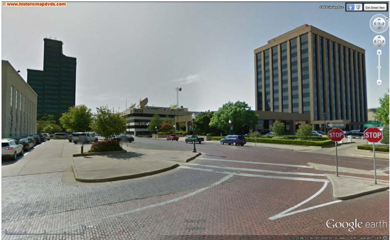
The second building of concern is the Regions building shown above. This structure has a height, to the roofline, of 142 feet, or 43.3 meters above ground level. From the K248CC antenna the closest distance to the Regions building is 158.7 meters. Additionally, the azimuth from the K248CC antenna spans the arc from 44 to 62 degrees true.
