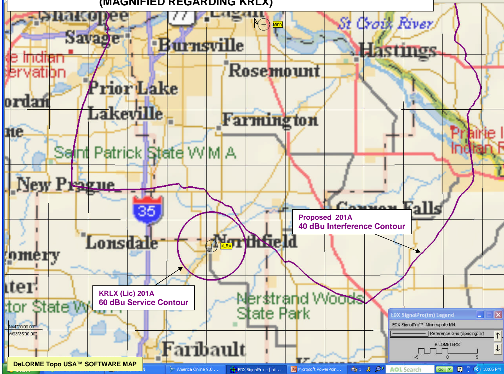
FIGURE E16.4—PROPOSED NEWPORT, MN 201A CO-CHANNEL PROTECTION (MAGNIFIED REGARDING KRLX)
