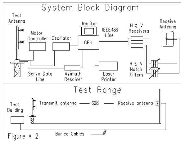
The antenna under test was operated in the transmitting mode and fed from a HP8657D signal generator. The frequency of the signal source was set at 105.9 MHz and was constantly monitored by a Rohde & Schwarz ESVD measuring receiver.
