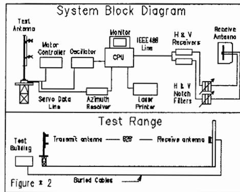
The antenna under test was operated in the transmitting mode and fed from a HP8657D signal generator. The frequency of the signal source was set at 89.7 MHz and was constantly monitored by a Rohde & Schwarz ESVD measuring receiver.
