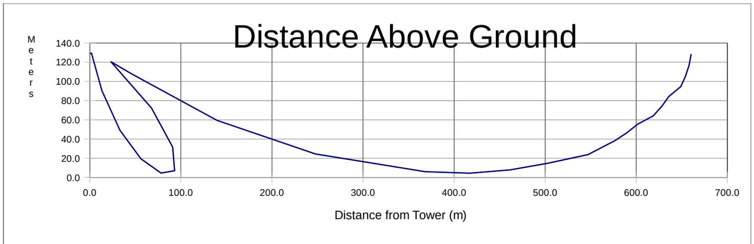
Location of 100.5 dbu contour above ground, versus distance from tower.
