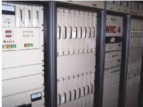
The solid state HPA used by WRC-TV, Channel 4, has an output power level of 52.5 kW.
