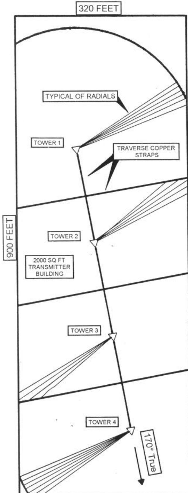
The proposed antenna system consists of 4 guyed towers each 59.7 meters (77.4°) tall, spaced 54 meters (70°) apart on a bearing of 170° true. The ground system will consist of 120 equally spaced #10 AWG copper wires 69.4 meters in length except where shortened by intersecting copper straps or property boundaries. A four inch copper strap will run from tower base to tower base
