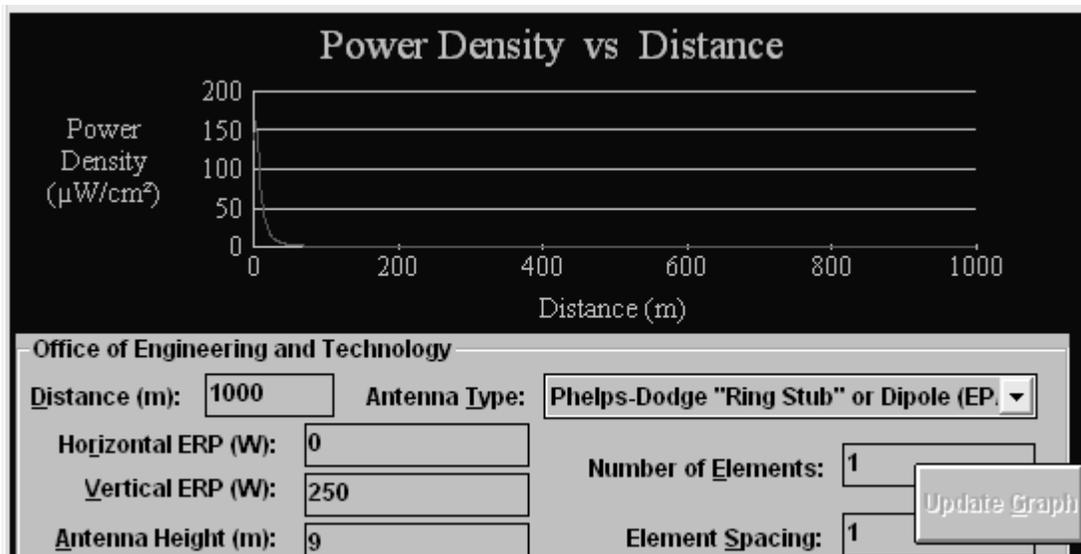
The Max Power Density was found to be  $161.647079150813 \mu\text{W}/\text{cm}^2$  at 2 meters.
