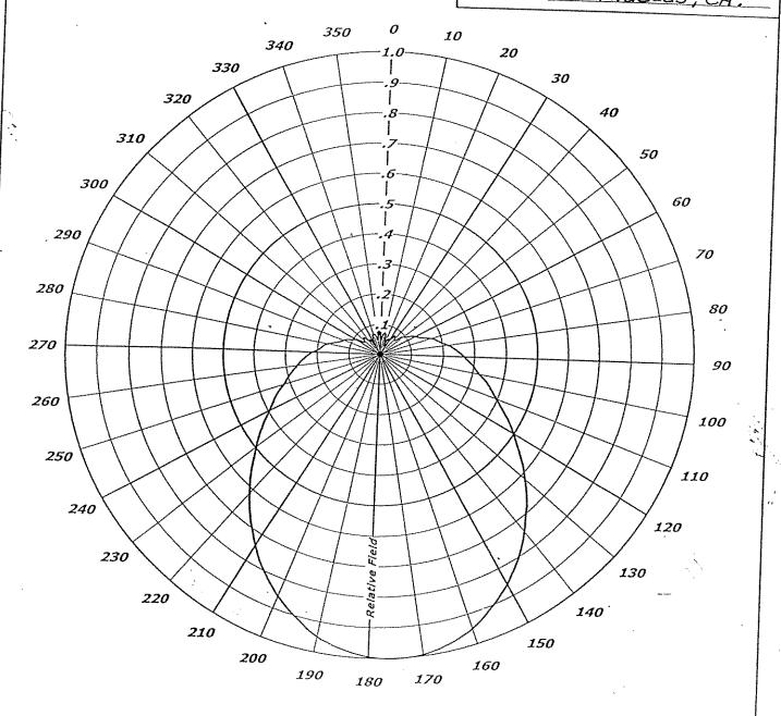
**EXHIBIT C** ELEVATION PATTERN CHISELH 1.0 Type: Directivity: dBdMain Lobe: Horizontal: .9 Beam Tilt: Polarization: HORIZONTAL Channel: ---LOS ANGELES, CA. Location: .8 .7 .6 .5 .4 .3 .2 . 1 10 **Above** Angle From Horizontal, Degrees Below ANDREW CORPORATION 10500 W. 153rd Street
