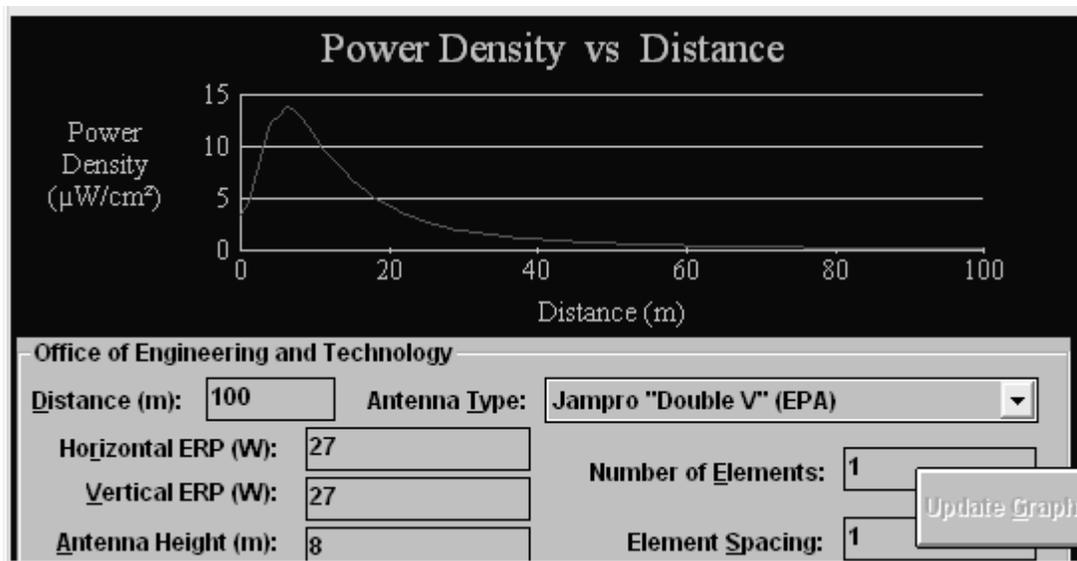
The Max Power Density was found to be  $13.7815294219406 \mu\text{W}/\text{cm}^2$  at 6 meters.
