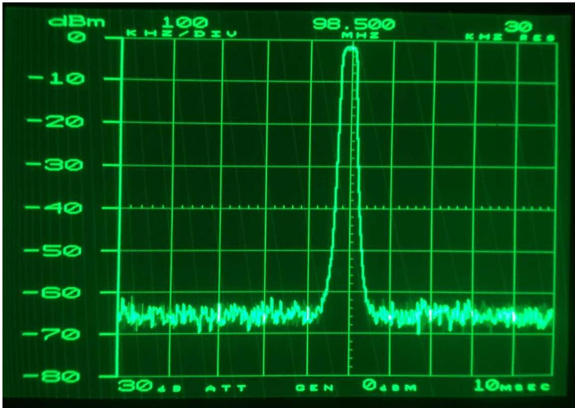
This is the spectrum analyzer showing emissions on 98.5 mHz (the translator K253AY. The marker shows a signal of -60 db from the K253AY reference signal.
