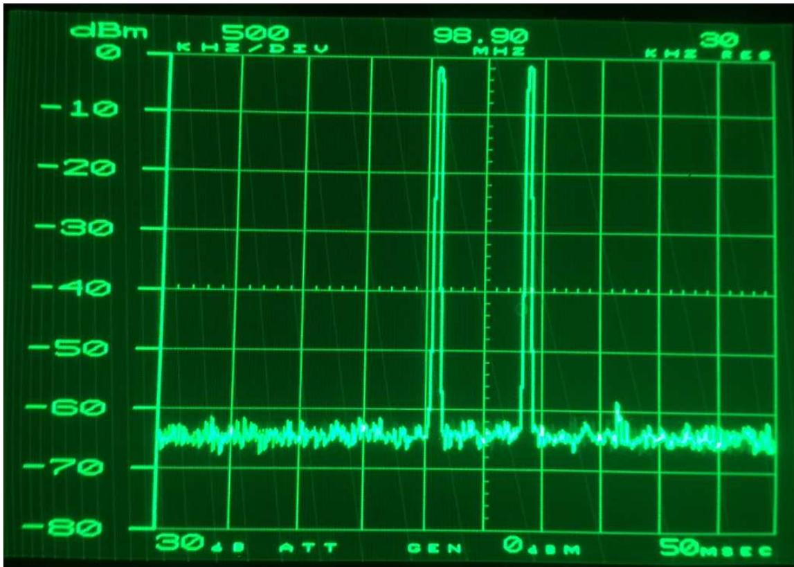
This is the spectrum analyzer showing emissions on 98.9 mHz (400 kHz removed from 98.5 mHz).
