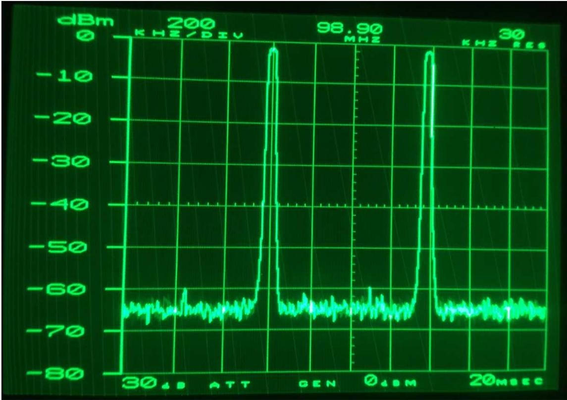
This is the spectrum analyzer showing emissions 400 kHz either side of 98.9 MHz).
