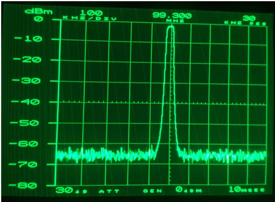
This is the spectrum analyzer showing the primary K257GA operation on 99.3 mHz. It should be noted that any spurious emissions are well below the FCC's maximums as specified in 73.317.
