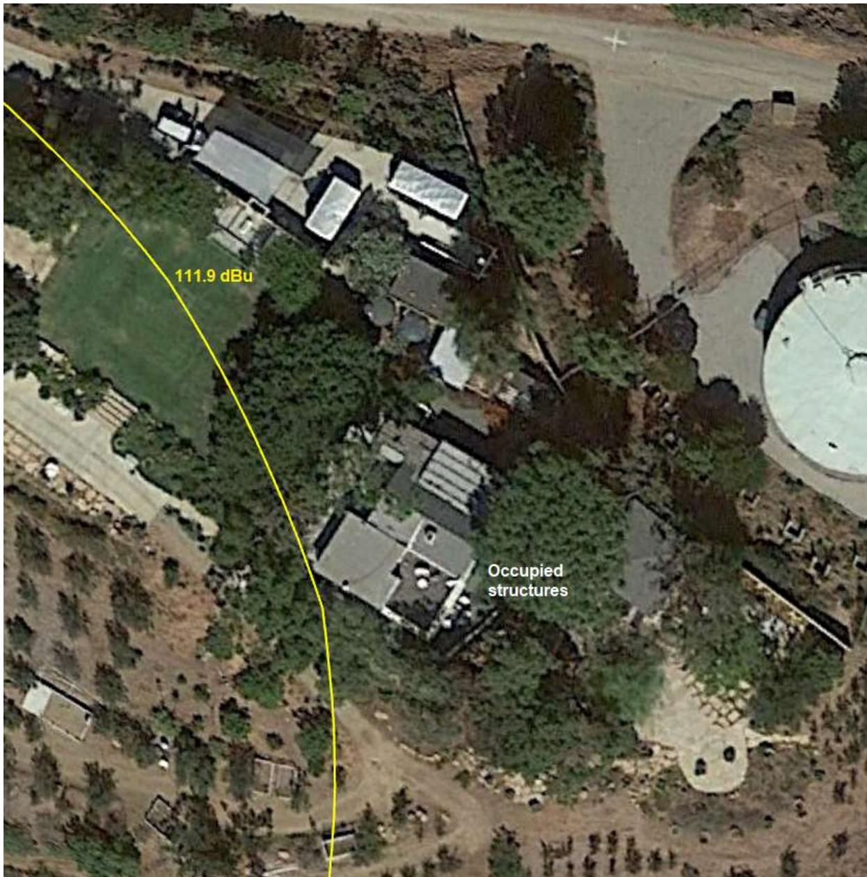
The occupied structures are outside of the 111.9 dBu interfering contour (overlap zone).
