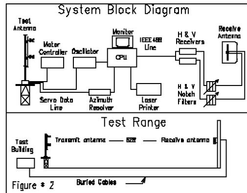
The antenna under test was operated in the transmitting mode and fed from a HP8657D signal generator. The frequency of the signal source was set at 99.3 MHz and was constantly monitored by a Rohde & Schwarz ESVD measuring receiver.
