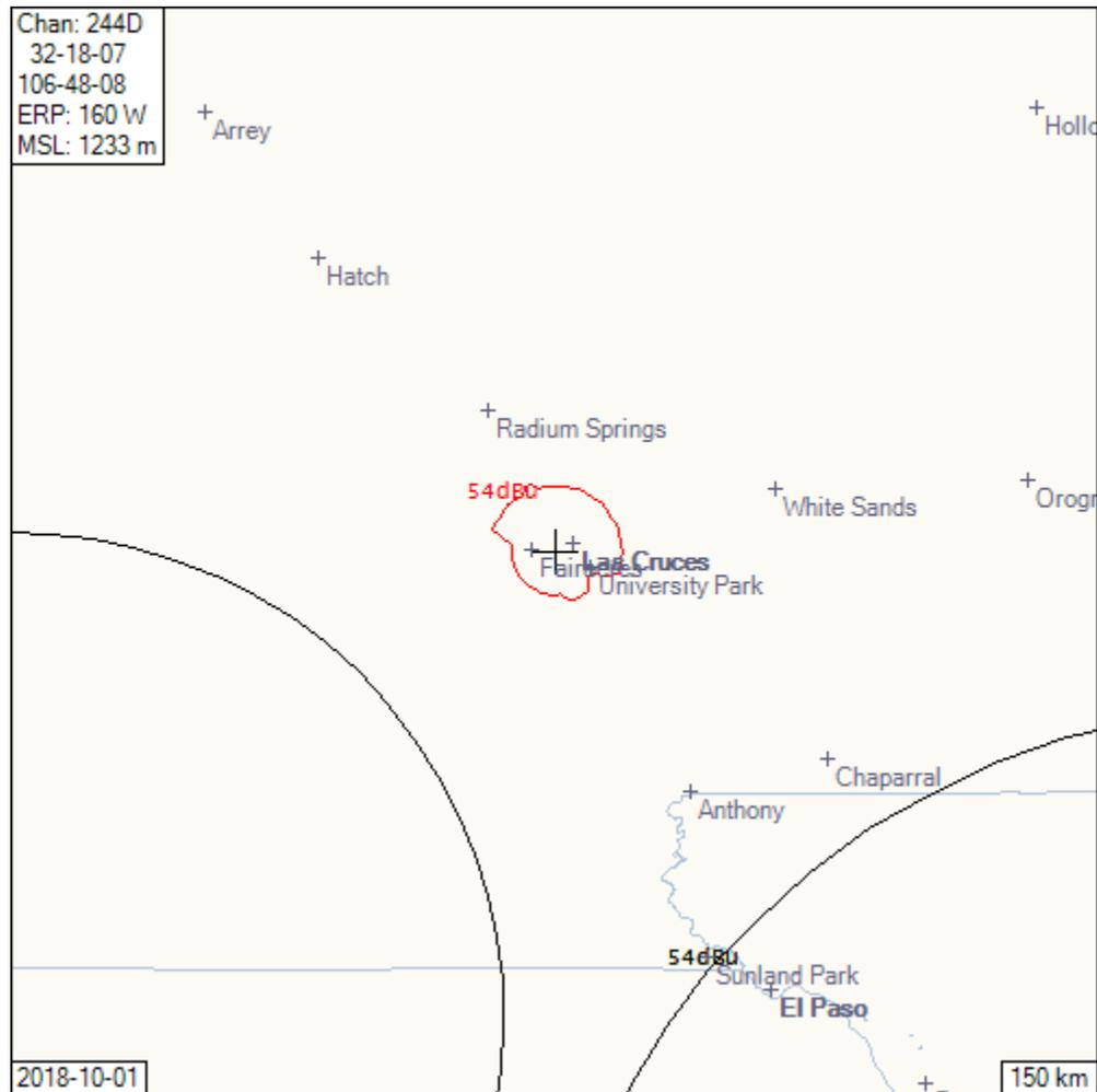
There is no overlap of the interfering contour with the protected contour of any first-adjacent station or proposal.
