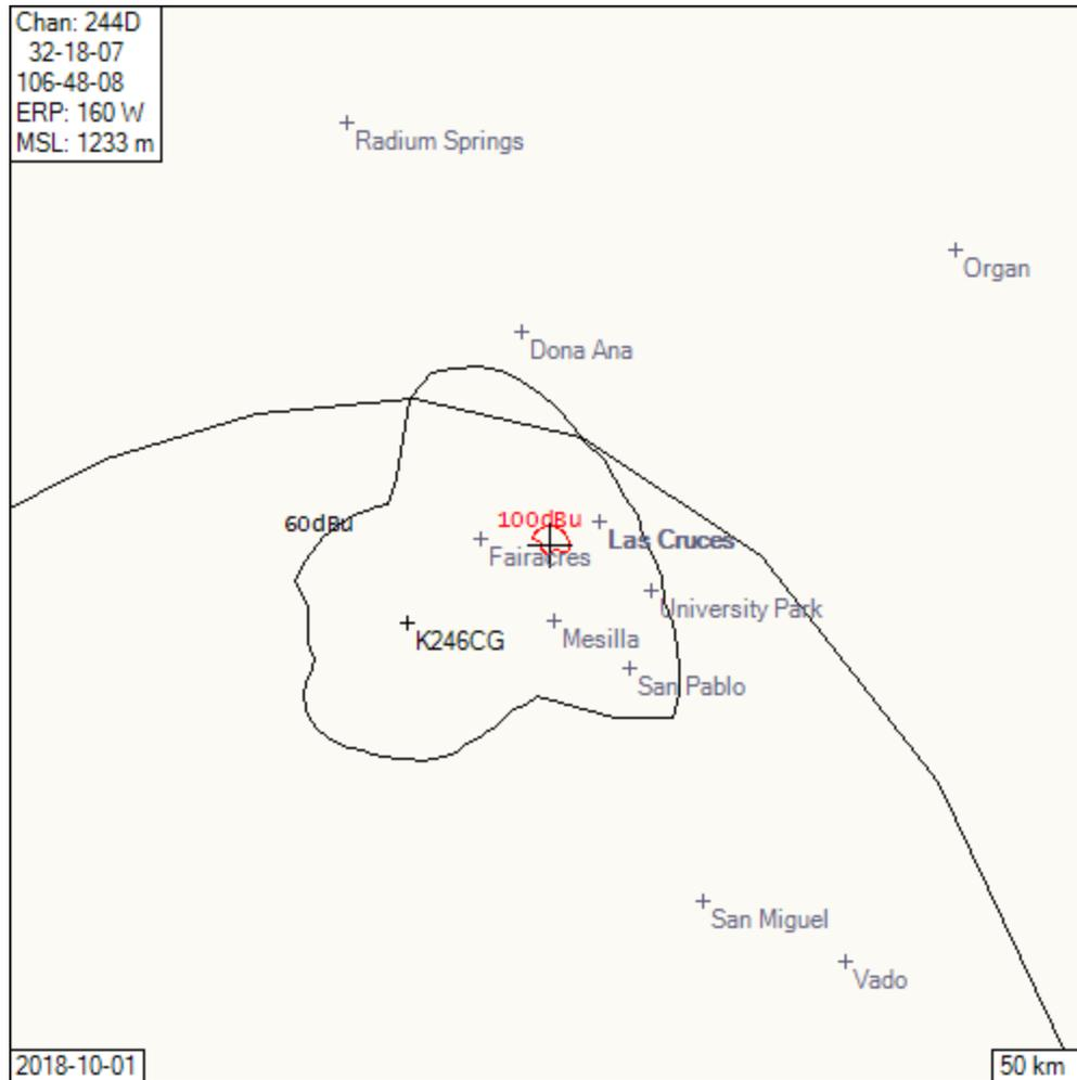
The proposed transmitter site is within the protected contours of K246CG and KHEY.
