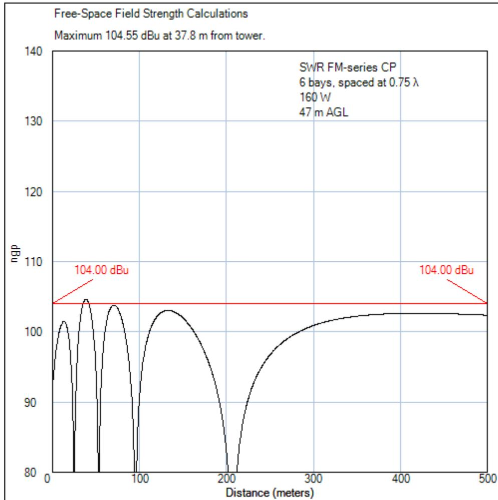
The above plot shows that the interfering signal on the ground will never reach the 104.0 dBu limit beyond about 50 m, but it would exceed the limit within 50 m.
