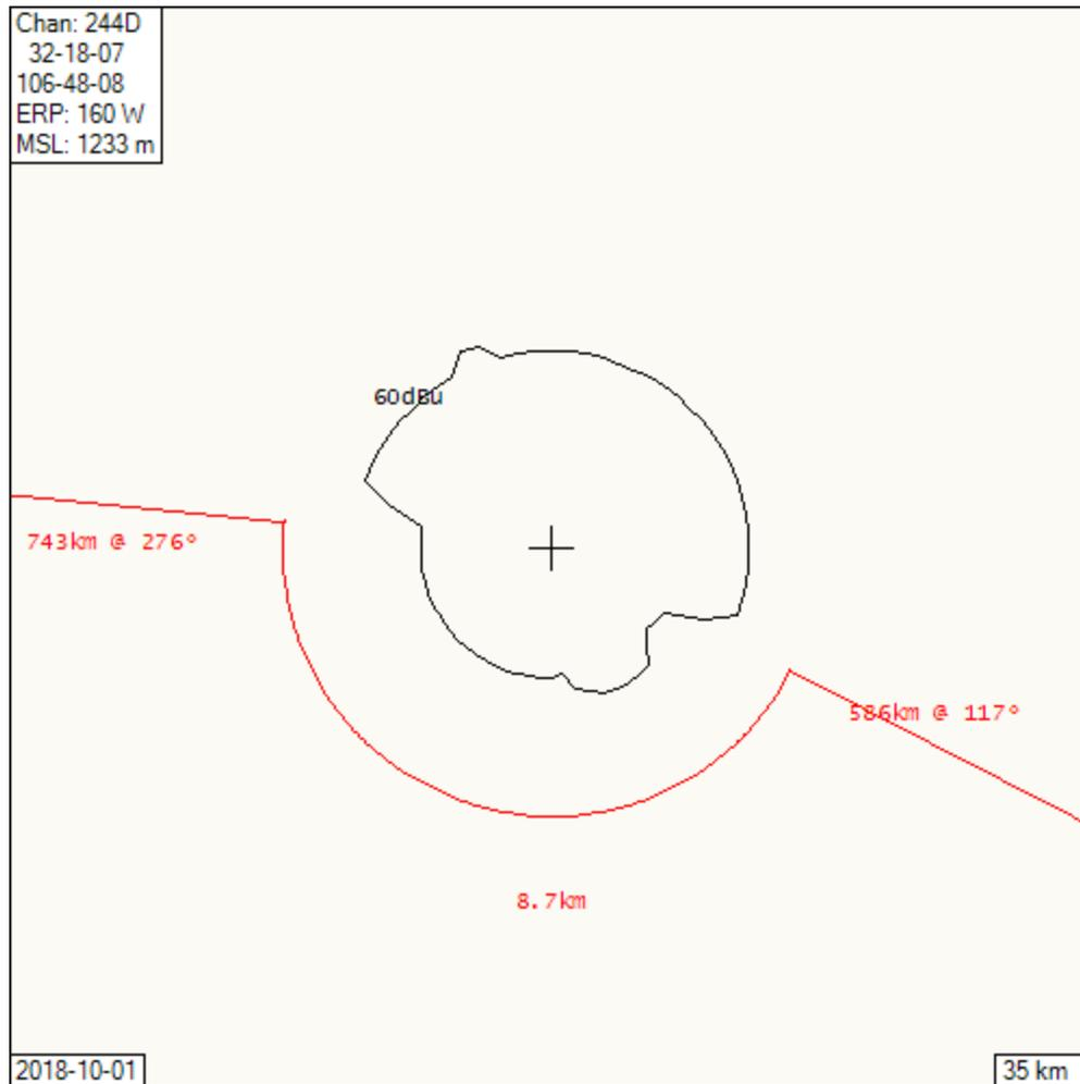
The protected contour does not exceed 8.7 km from 117° clockwise to 276°.
