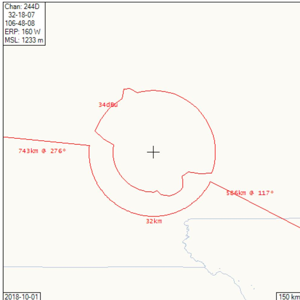
The interfering contour does not exceed 32 km from 117° clockwise to 276°.
