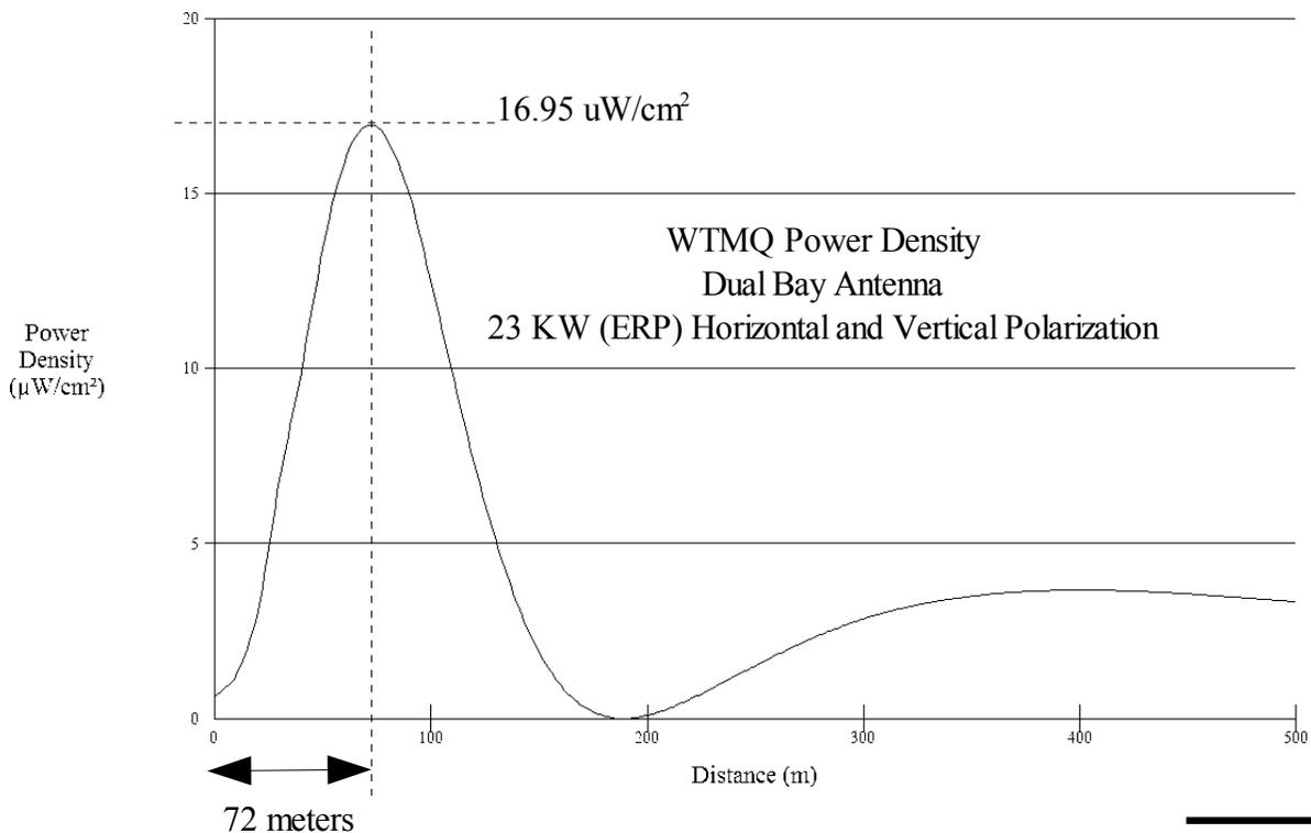
Occupational exposures shall be precluded by decreasing power, or suspending operations whenever personnel will be required to climb to areas with electromagnetic fields approaching the MPE limits of the ANSI Standard.
