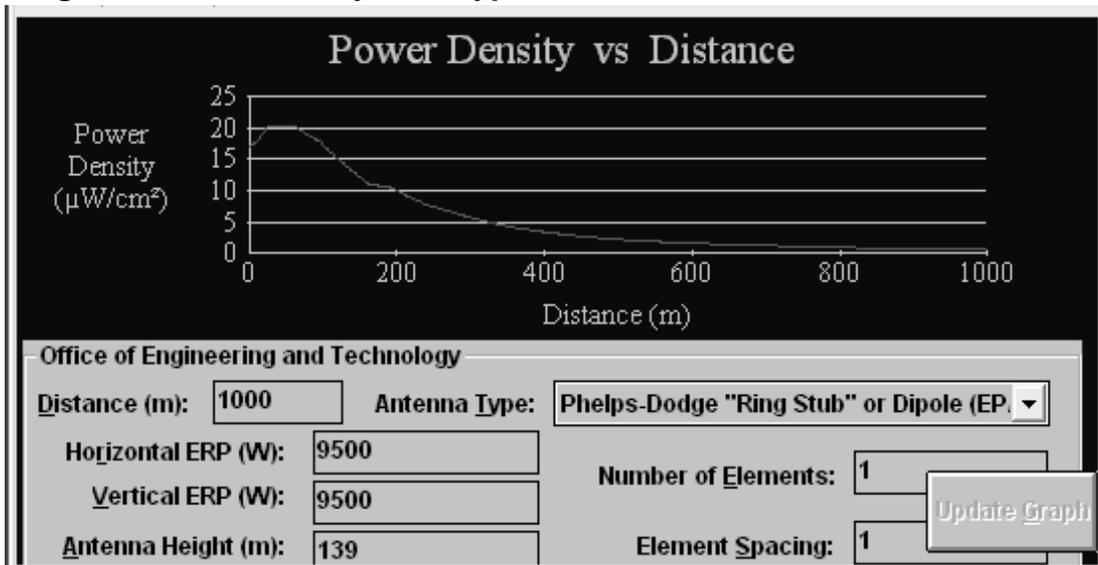
The Max Power Density was found to be 20.3505615021933  $\mu\text{W}/\text{cm}^2$  at 38 meters.
