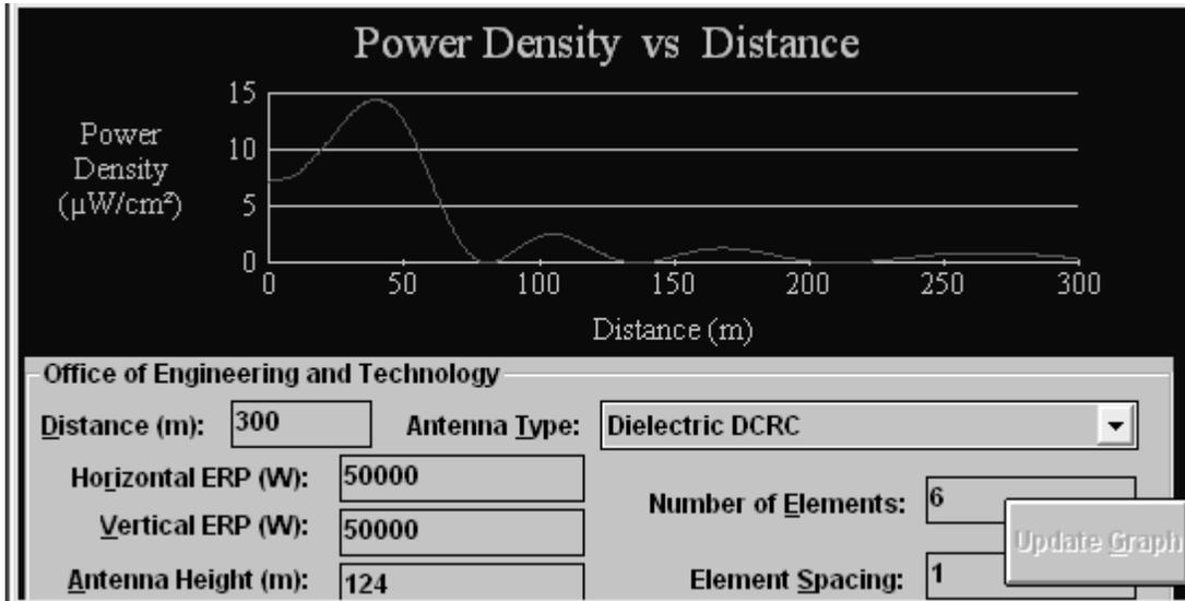
The Max Power Density was found to be 14.4660631187905  $\mu\text{W}/\text{cm}^2$  at 39.6 meters.
