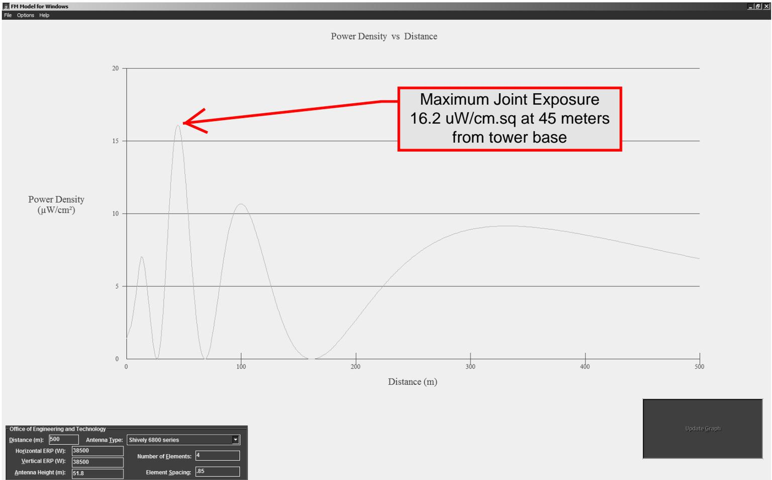
Channels 228C0 with 20 kW (KWES) & 274C1 with 18.5 kW (New CP) will be co-located on same tower using separate 4 bay Shively antennas with 0.85 wavelength spacing.
