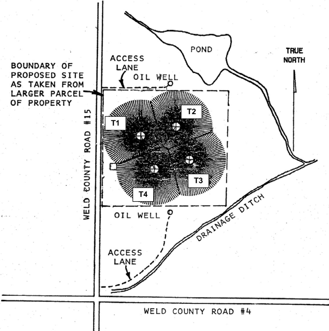
GROUND SYSTEM SHALL CONSIST OF 120 EQUALLY-SPACED #10 SOFT-DRAWN COPPER WIRE RADIALS SURROUNDING EACH TOWER. RADIALS ARE TO BE 323 FEET (90° @ 760 KHZ.) LONG EXCEPT WHERE SHORTER DUE TO INTERSECTION WITH RADIALS OF ADJACENT TOWERS. INTERSECTING RADIALS WILL BE BONDED TO TRANSVERSE STRAPS (HEAVY LINES SHOWN). IN ADDITION, 120 SHORT 50-FOOT RADIALS SHALL BE INTERSPERSED AMONG THE PRIMARY RADIALS OF EACH TOWER. ALL CONNECTIONS SOLDERED
