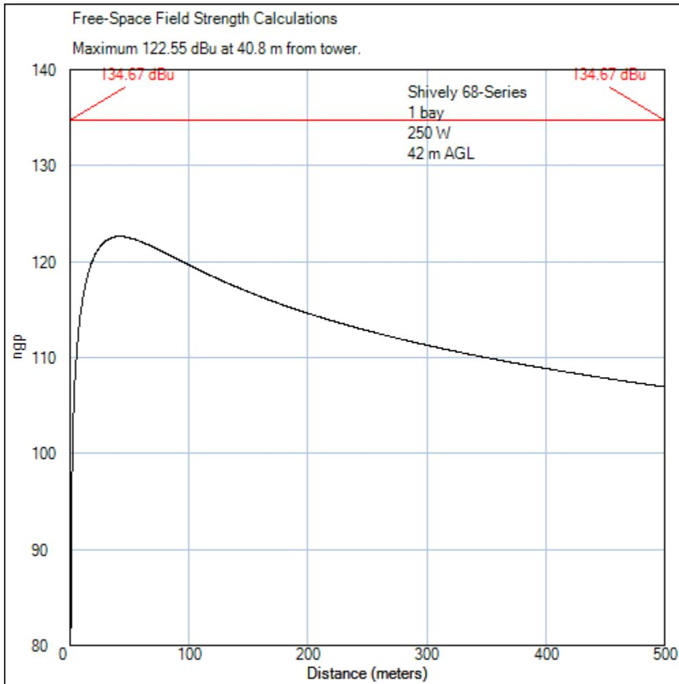
This plot shows free-space signal strength 2 m above ground level (44 m actual height, less 2 m). The interfering signal is more than 12 dB below the limit.
