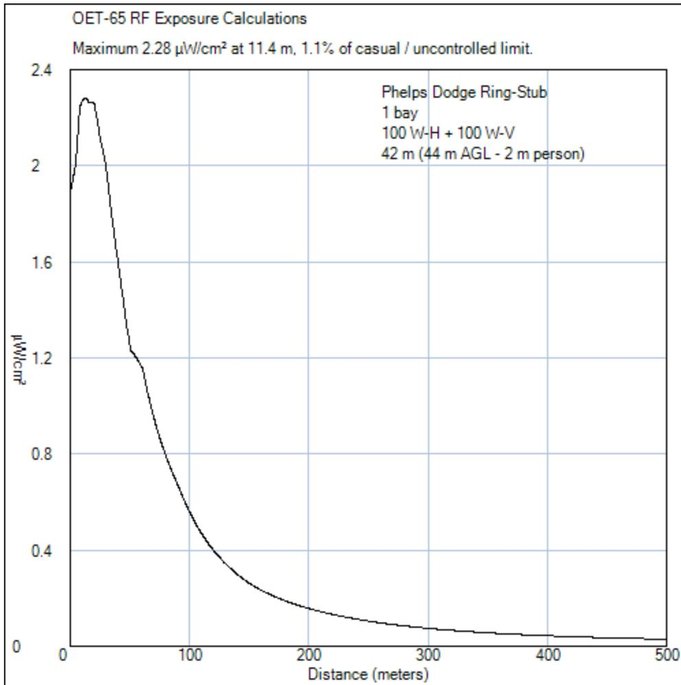
Assuming one bay of the worst-case antenna (OET Type 1 Ring-Stub), the maximum exposure would be about 1% of the limit for casual / uncontrolled exposure.
