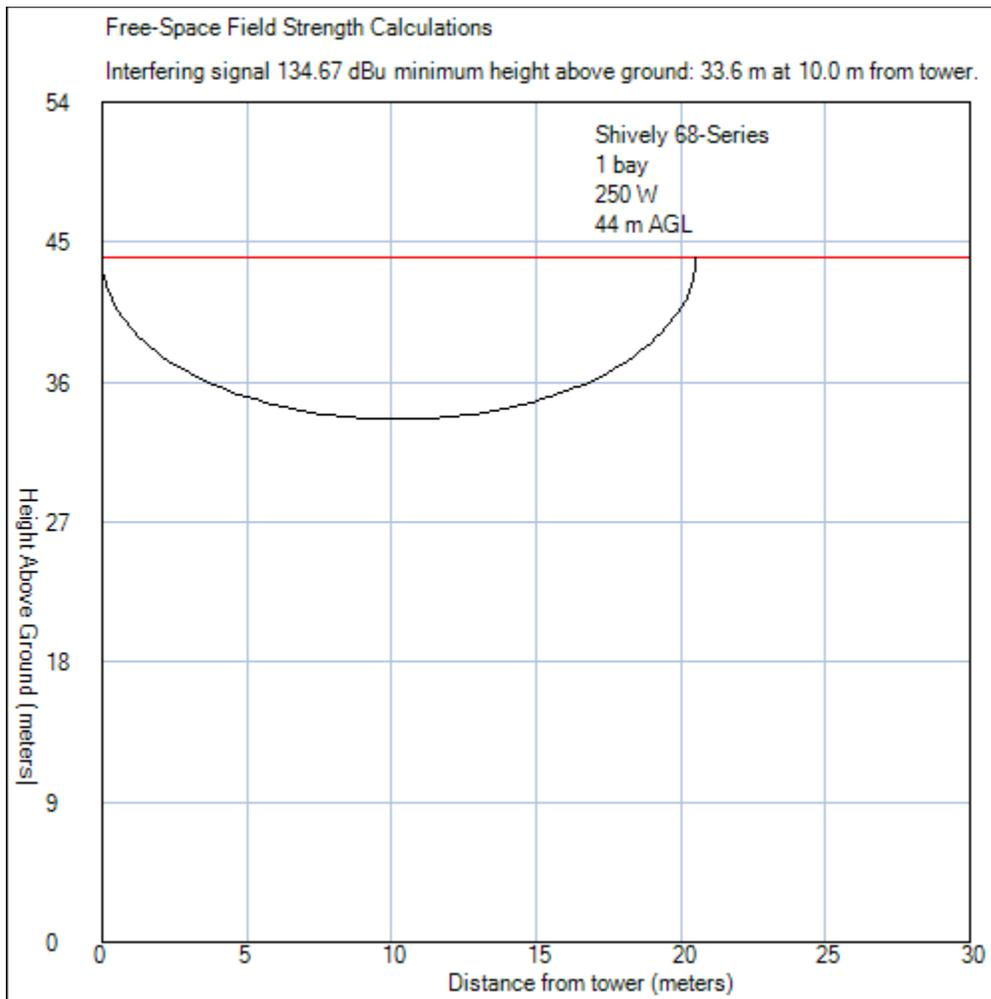
This plot shows the height of the 134.67 dBu free-space interfering signal above ground. It is at least 33 m above the ground. The maximum distance to the interfering signal is 50.0 m. No tall buildings exist in the vicinity.
