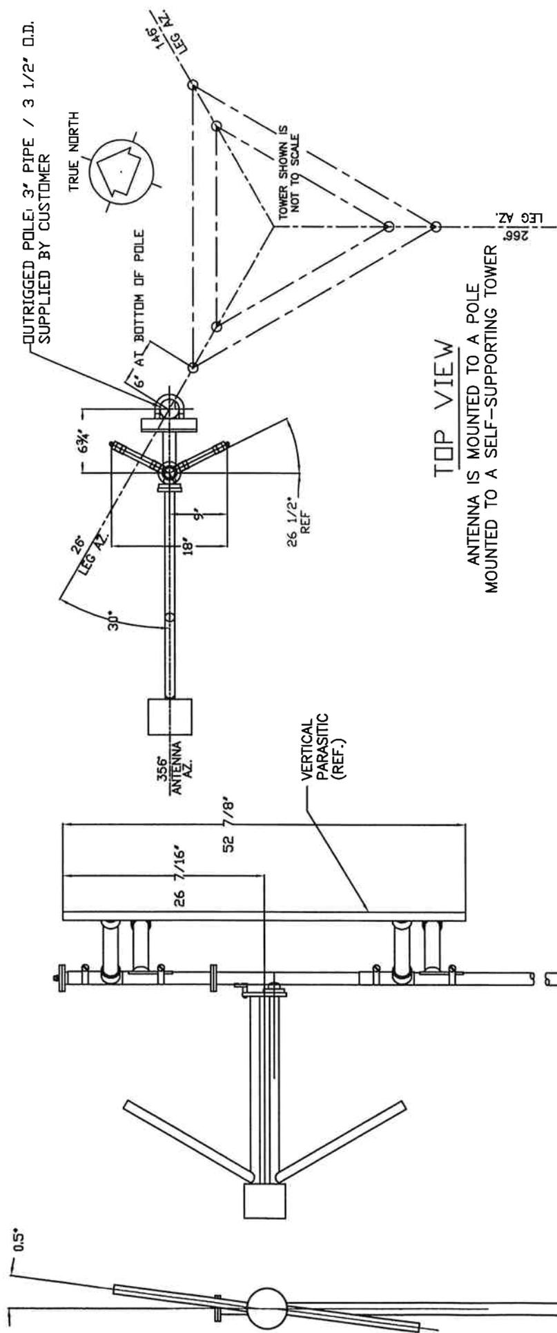
OUTRIGGER POLE, 3" PIPE / 3 1/2" O.D. SUPPLIED BY CUSTOMER
