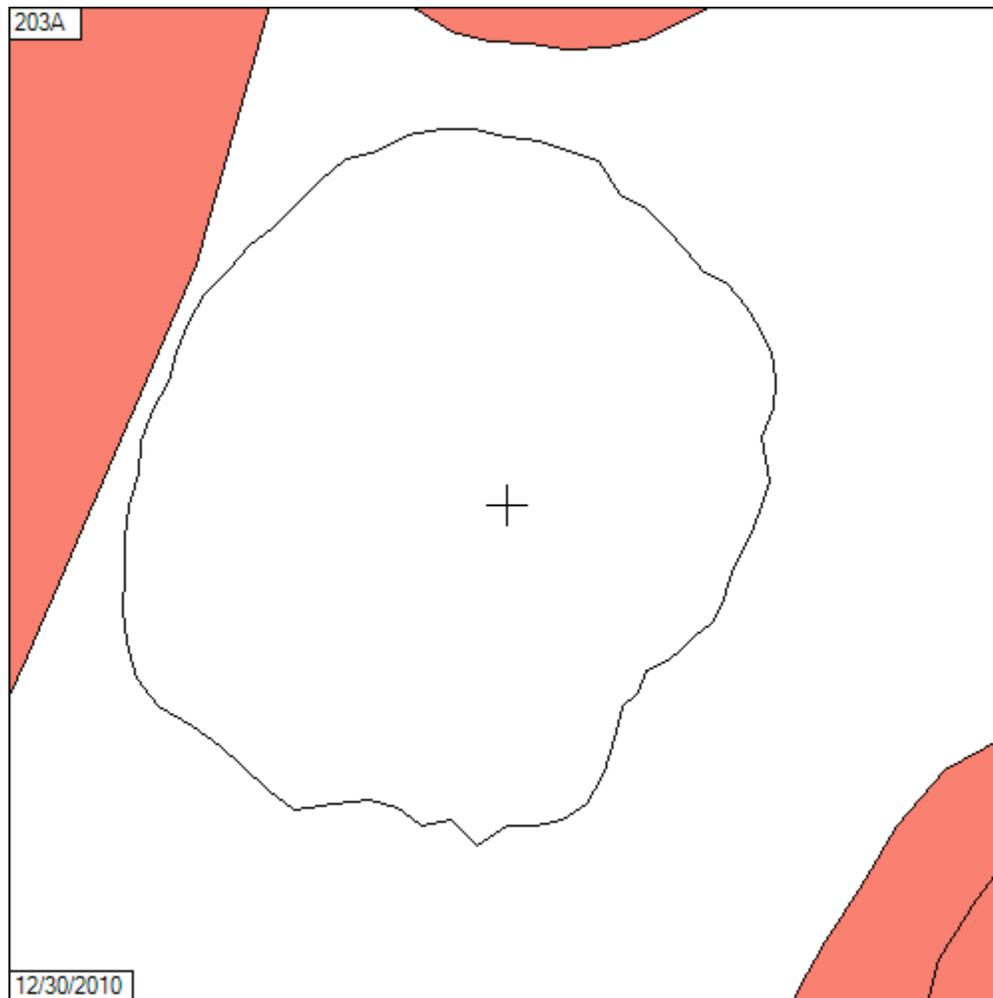
This close-up shows that no prohibited overlap occurs between the proposed 60 dBu f(50,50) (shown in black) and the inbound 40 dBu f(50,10) interference from WFCR (black filled with salmon).
