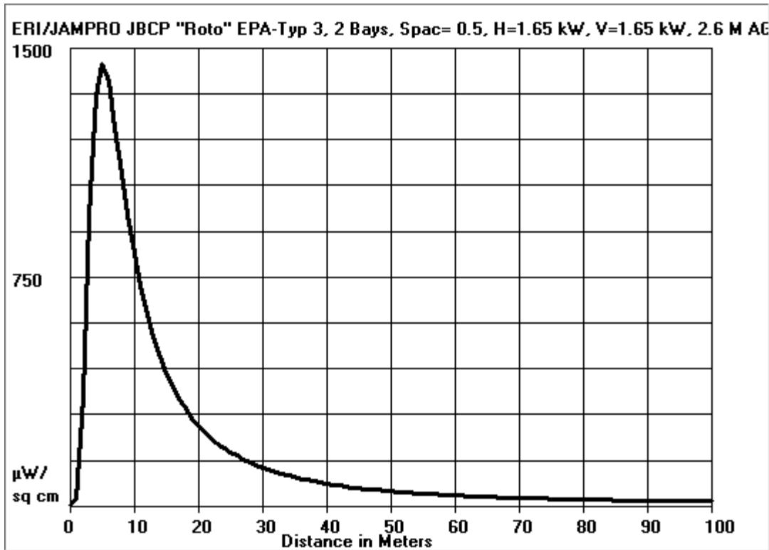
RF Power Density at Head height from the roof level at 8.7 meters from the antenna center of radiation
