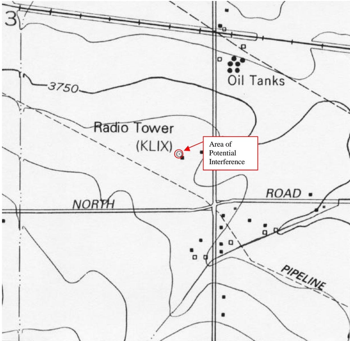
This is an enlarged section of the relevant USGS map FILER, IDAHO showing the F(50,10) 128.25 dBu contour overlap area. The interference zone is entirely encompassed by the F(50,50) 88.25 dBu contour of the 2nd adjacent FM station KEFX.
