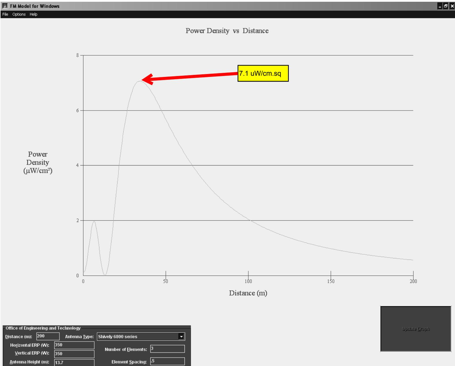
The above plot is for a 3 bay half-wave Shively antenna. The RF contribution at 2 meters above the ground will be less than 8 uW/cm.sq. This is well below even the public exposure limit of 200 uW/cm.sq.
