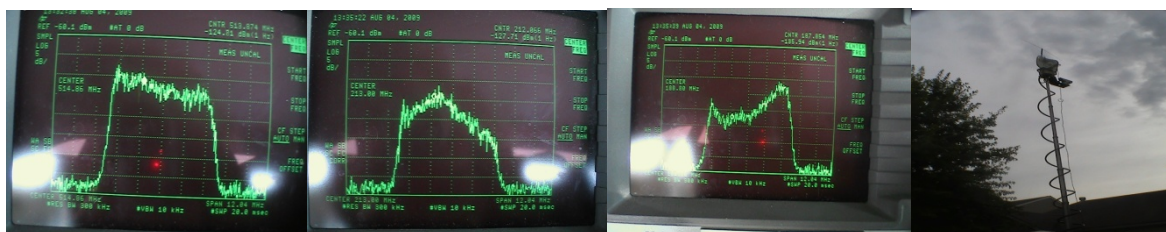
8-4 5:45 PM Consumer Dipole at 30' (mast up and antenna rotated for maximum on each signal)
