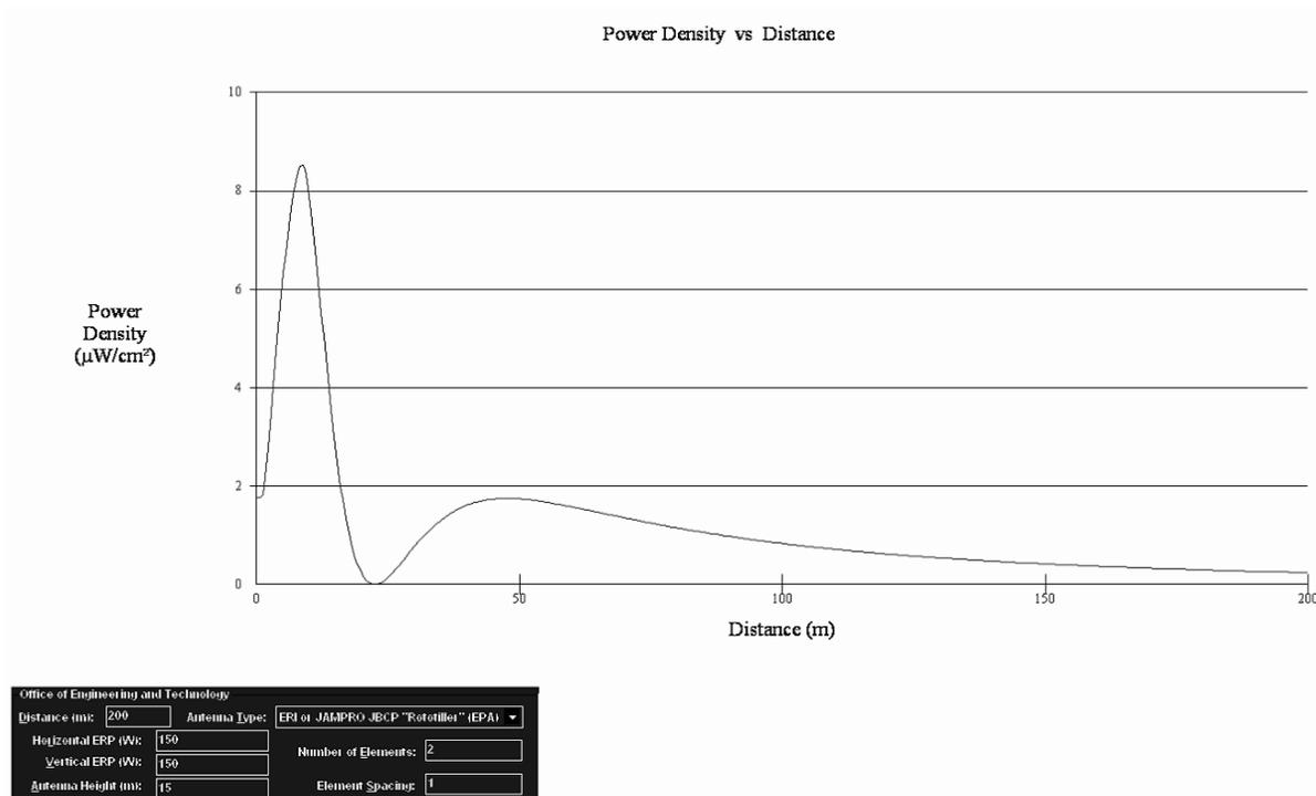
The above graph is for the proposed Goldfield application. The study is from the FCC FM-Model program to demonstrate compliance with ANSI and show that there will be no human radiation exposure with the proposed facility.
