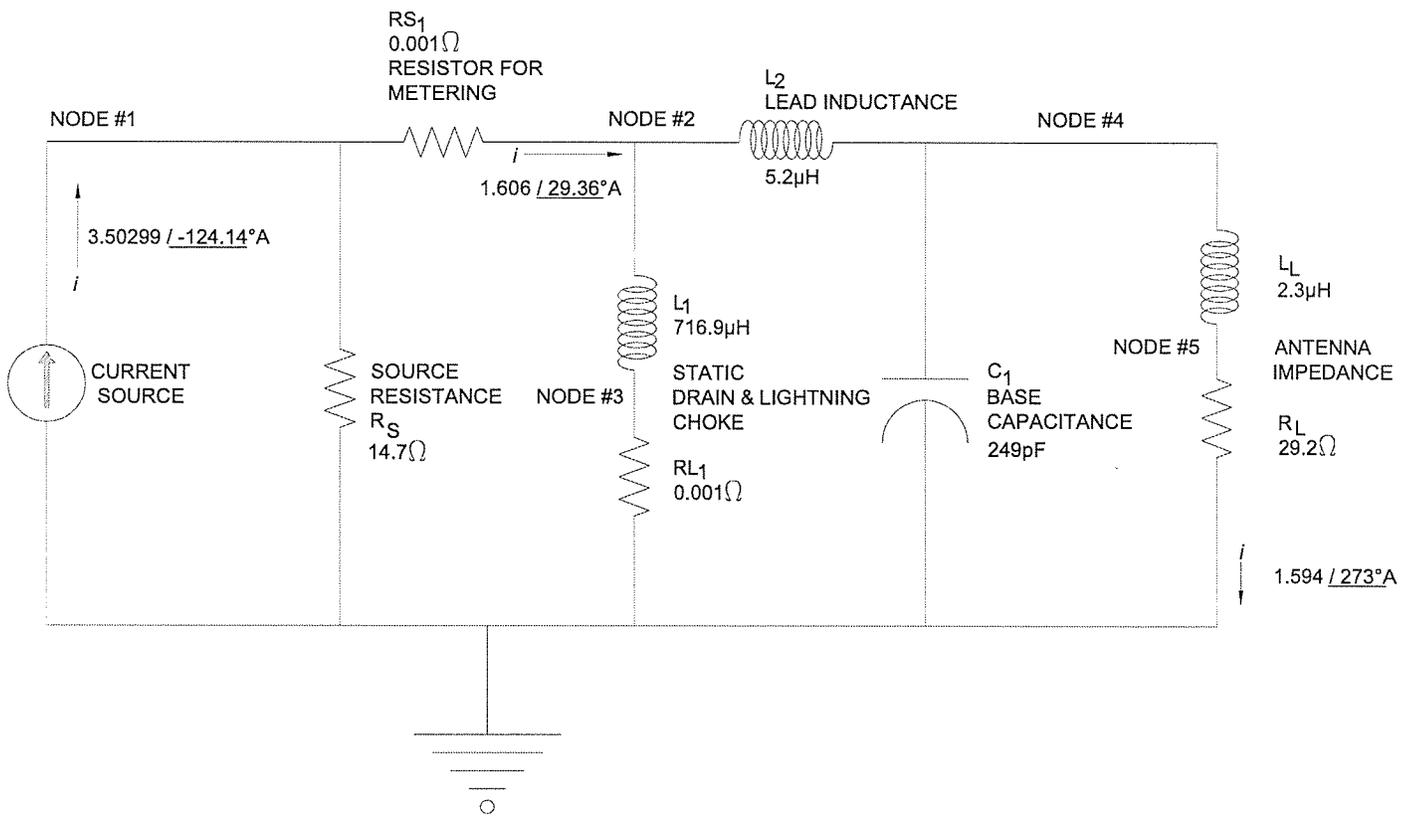
*Calculated Antenna Monitor Parameters*
