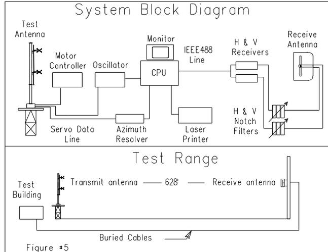
motor drive and a US Digital angle position indicator. The resolution of this angle position indicator is one-hundredth of a degree.
