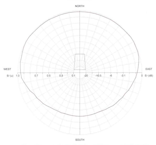
0.0° depres. (Total antenna), Gain (dBd): -2.9 ERP T.max (KW): 0.519 ERP E.max (KW): 0.403
