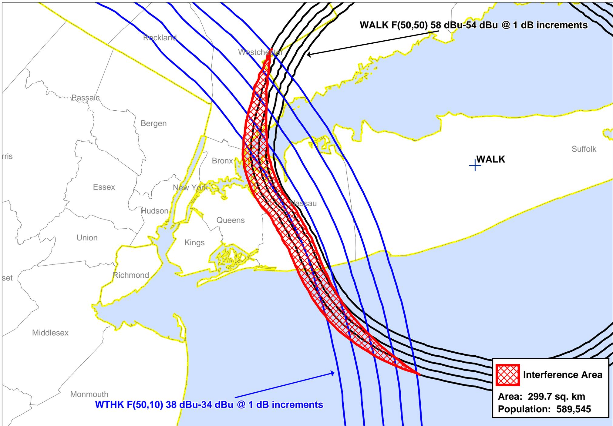
**WALK & WTHK (Licensed) [Interfering] Desired/Undesired Interference Study**
