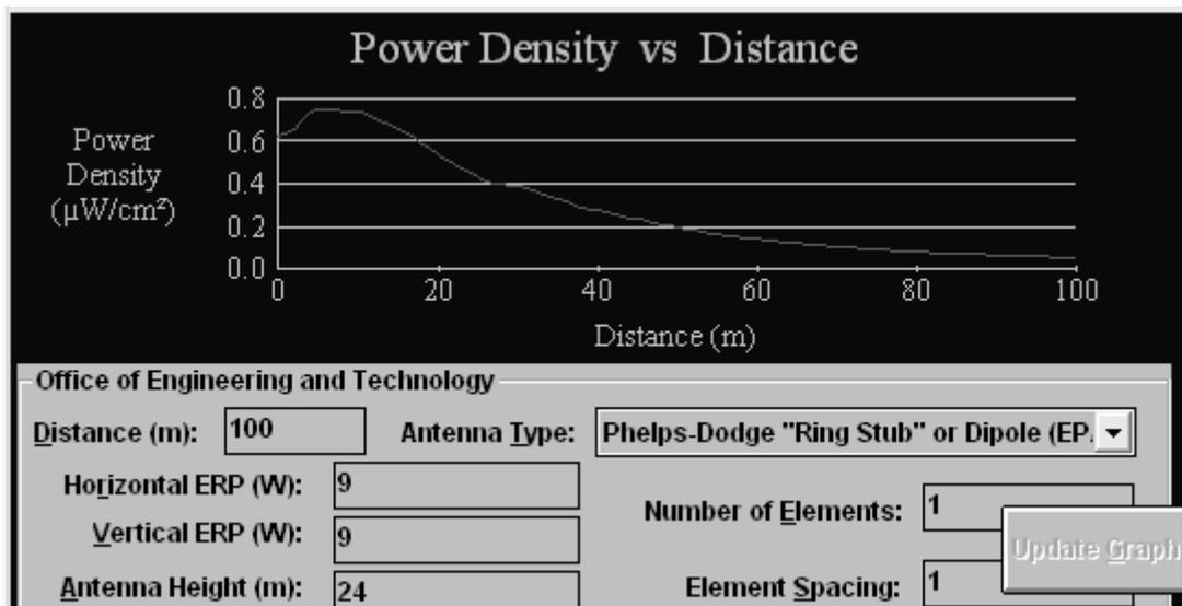
The Max Power Density was found to be .747726011552901  $\mu\text{W}/\text{cm}^2$  at 6 meters.
