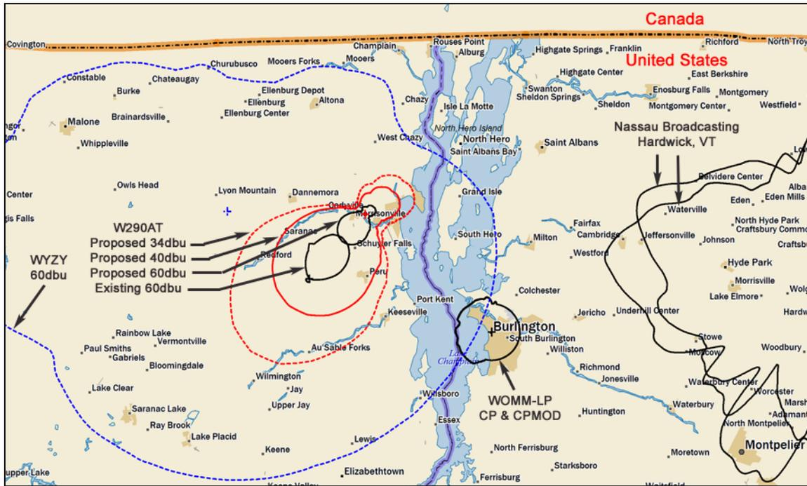
On the above map, red contours represent  $f(50,10)$  interfering signals, black contours represent 60dbu  $f(50,50)$  protected contours, and the blue dashed contour represents the 60dbu  $f(50,50)$  contour of WYZY, Saranac, NY, the primary station.
