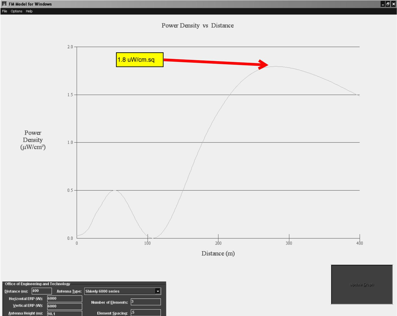
The above plot is for a 3 bay half-wave Shively antenna. This antenna will be used by the proposed operation of WAFC-FM with a 6 kW ERP. The RF contribution at 2 meters above the ground will be less than 2 uW/cm.sq or 0.2% of the controlled limit. This is well below even the public exposure limit of 200 uW/cm.sq.
