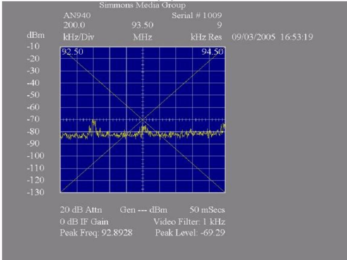
Measured Intermodulation Product with KJQN (FM) 103.1 MHz 2 X 97.5 – 103.1 MHz=91.9
