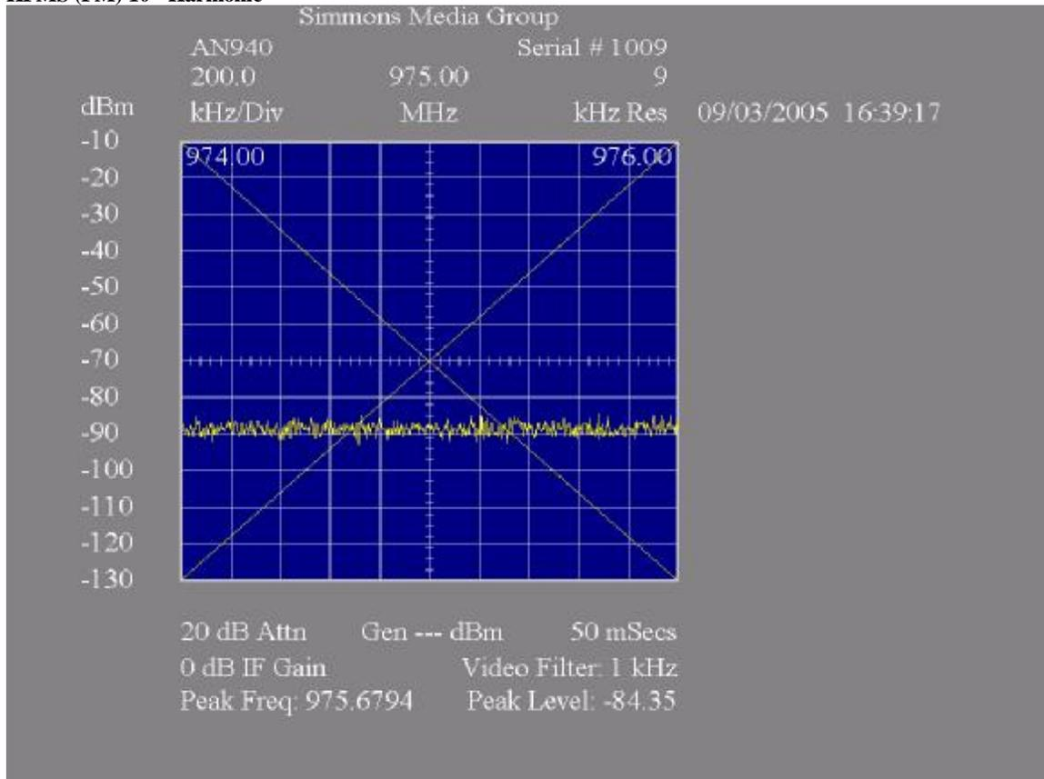
Measured Intermodulation Product with KEGA (FM) 101.5 MHz 2 X 97.5 – 101.5 MHz=93.5
