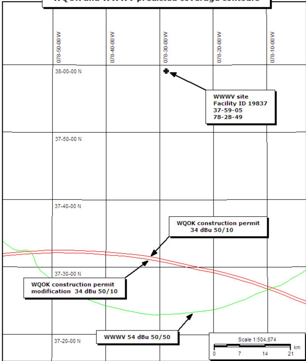
**Interference to WWWV from the instant construction permit modification proposal is contained within area currently receiving interference from the facility authorized by the construction permit, in compliance with Section 73.213 (a)**
