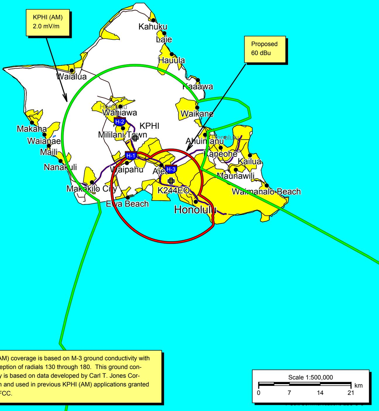
KPHI (AM) coverage is based on M-3 ground conductivity with the exception of radials 130 through 180. This ground conductivity is based on data developed by Carl T. Jones Corporation and used in previous KPHI (AM) applications granted by the FCC.
