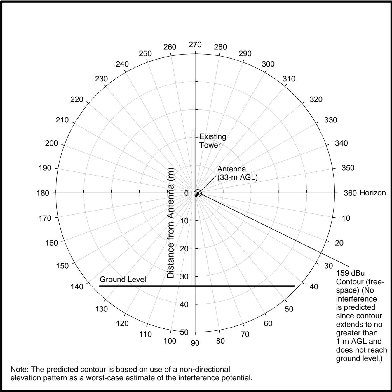
**VERTICAL PLAN VIEW OF 159 dBu CONTOUR
