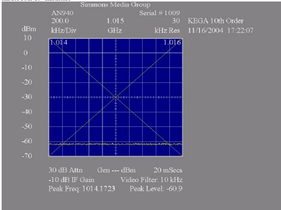
Measured Intermodulation Product with KPEB (FM) 103.1 MHz 2 X 101.5- 103.1 MHz = 99.9MHz
