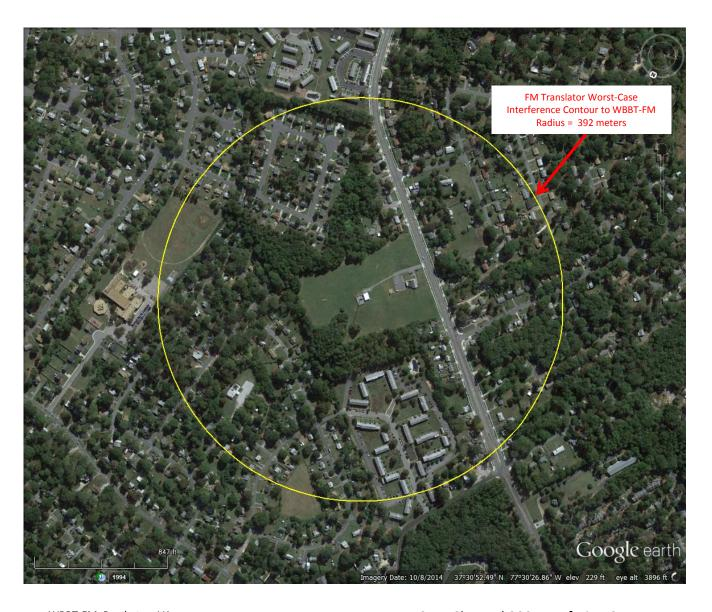
WBBT-FM, Powhatan, VA Ch. 297A, 1.4 kW ERP, 207 m HAAT FCC File No. BLH-20110525ABA
