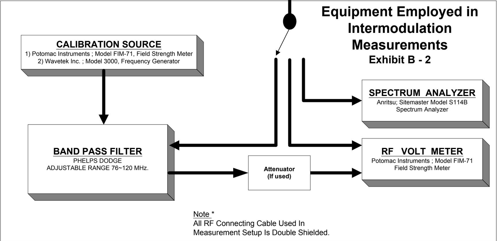
Broadcasting Scheme and Equipment Employed in Intermodulation Measurements
