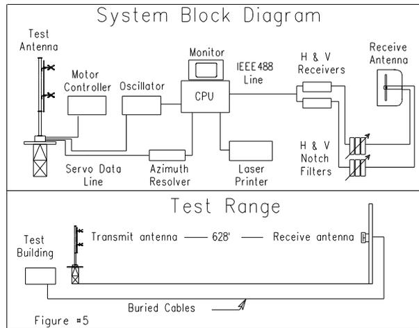
equipped with a motor drive and a US Digital angle position indicator. The resolution of this angle position indicator is one-hundredth of a degree.
